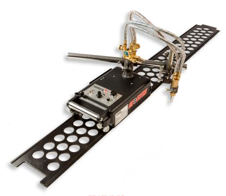
The dart CG1-30 is a light weight, portable power-driven flame cutting machine with plasma torch outfitting capabilities. The straight-line cutter is exceptional for cutting long plates, beveled angles, and circular cuts.
